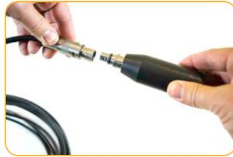
After attaching cable to instrument, connect cable to the TROLL Com.
