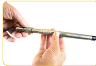
Press cable into instrument connector.
