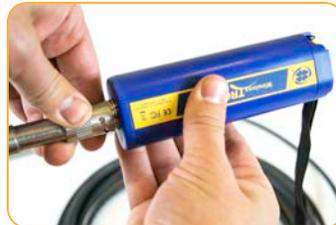
Push and twist to lock cable to communication device.
