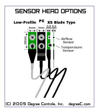
*Fig. 1: Low-Profile (left), PC (center), and XS Sensor Heads.*
