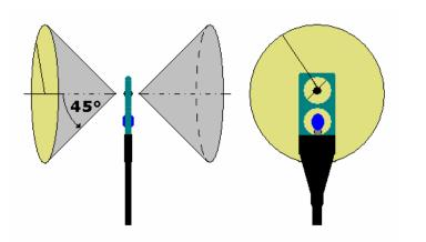
*Fig. 3: Airflow acceptance angle for PC and Low-Profile sensor heads as recommended by AccuSense.*
