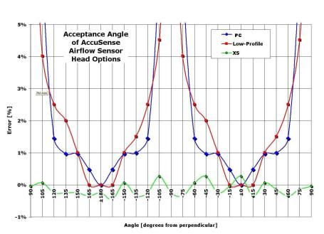
*Fig. 2: Accuracy of AccuSense sensors vs. angle from perpendicular of oncoming airflow.*
