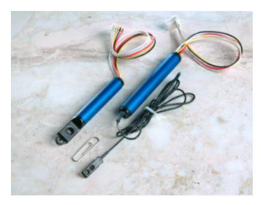
Theory of Operation: The AccuSense F900 Sensors use thermal anemometer technology, which measures heat loss from a heated device. Two thermistors on the sensor head detect airflow and ambient temperature simultaneously. The airflow reading is then compensated for temperature within the specified calibration range, linearized, and made available at the output. Each sensor is individually calibrated, which makes the F900 fully interchangeable.
