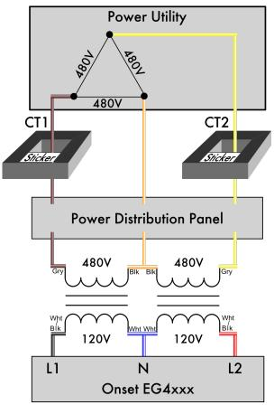
Transformers: 2x Functional Devices TR50VA008 480V/120V 50VA
