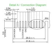
Contact Pins for DIP-28 wide IC socket 28-pin or for soldering
