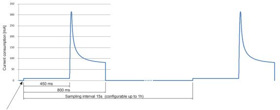
First reading occurs 5...15 seconds after power on, for details see Application Note at www.epluse.com/ee894.
