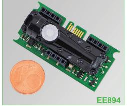
An optional kit for the E2 interface facilitates easy configuration of the module and the adjustment of the  $CO_2$ , RH, T and p measurement. The  $CO_2$  measurement interval can be set according to the application requirements; by this the average current consumption can be reduced to 420  $\mu$ A, ideal for battery-operated devices.
