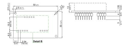
Detail B / Connection Diagram:
