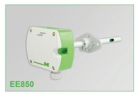
Installed into a duct, a small amount of air flows through the divided probe to the  $CO_2$  sensing cell located inside the transmitter enclosure and back into the duct. The RH and T sensing elements are placed inside the probe.
