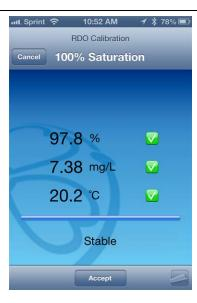
6. Remove the sponge and add fresh sodium sulfite solution to the fill line. Place the instrument into the calibration cup, and tap **Start**.
