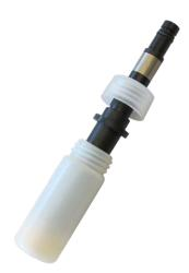
6. Place the sensor tip in the buffer and tighten the cap to prevent the glass bulb from drying.
