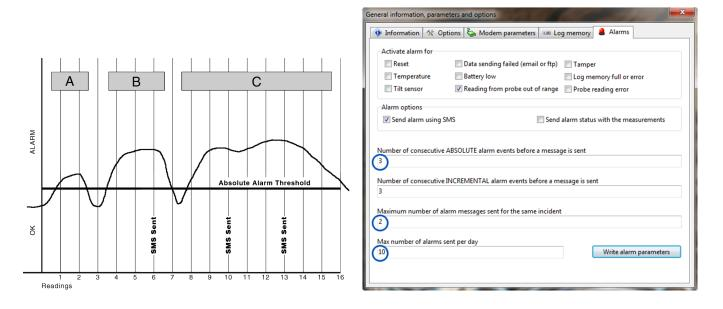
In Absolute Mode, alarms and warnings occur when a measurement value is less than the minimum threshold value or greater than the maximum threshold value.
