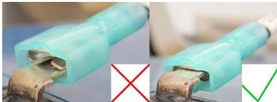
3. Plug the red (positive) leads into the red battery terminals. Ensure that the terminal does not sit between the lead clip and the plastic sheath, but that the lead clip encompasses the battery terminal.
