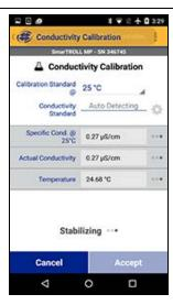
Check your bottle of calibration standard to determine the reference temperature. If necessary, tap the drop down list and select the appropriate reference temperature for the calibration.
