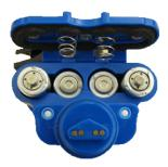
4. Close the cover and slide the lever to lock the compartment.
