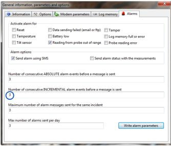
In Incremental Mode, alarms and warnings occur when the difference between two consecutive measurement values is less than the minimum threshold value or greater than the maximum threshold value. This difference means the alarm threshold is a slope instead of a fixed value.
