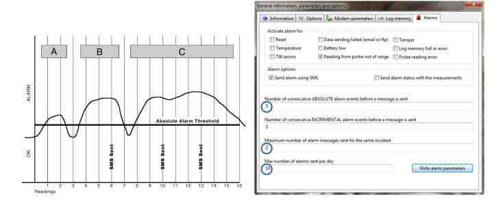
In Absolute Mode, alarms and warnings occur when a measurement value is less than the minimum threshold value or greater than the maximum threshold value.
