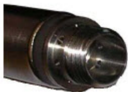
Nose cone removed - do not touch the exposed diaphragm
