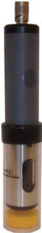
Figure 5.2 Calibration chamber with water-saturated sponge.
