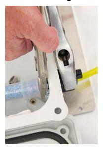
Unscrew the nut from the N-female to RP-SMA connector. Remove the star washer.
