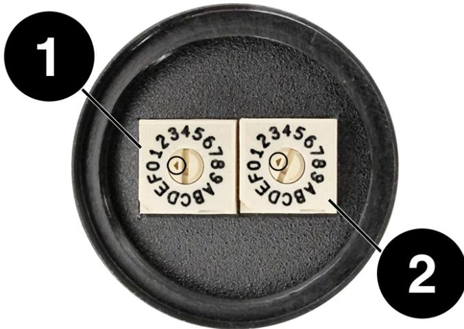
Figure 1.8 Radio addressing dials (arrows point to address)
