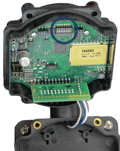
Figure 1.3 Radio DIP switch location
