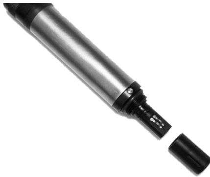
Figure 4.7 RDO Titan Probe and RDO Classic Sensor Cap with electrical contacts aligned
