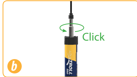
Attach opposite end of cable to the Aqua TROLL 500.
